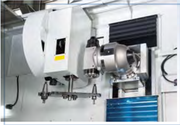
Vertical tool change with 24 stations swing arm type
