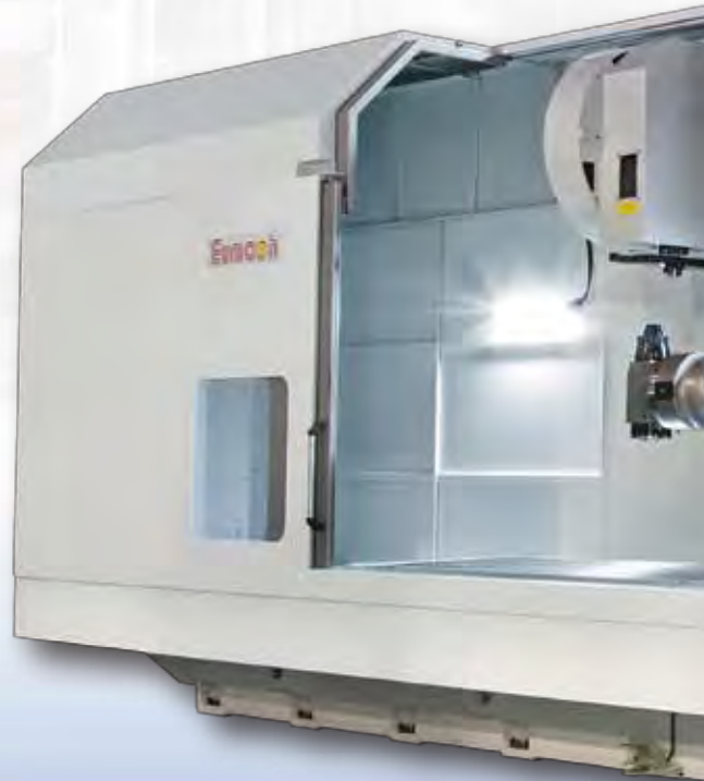
▶ FBE-4000 with 4000 / 1000(1250) / 950(1500)mm travel & optional top closed sliding roof full splash guard & auto. orthogonal milling head & 24 ATC
